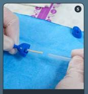
Remove tip cover and place exposed tip on blue wrap
